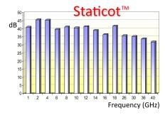
Polyester/Cotton blended with micro-fine 8µm stainless steel fibers creates a low cost, tough fabric similar to khaki. Perfect for grounding applications. **1000 Ohm per sq** on the surface, so it is great for
